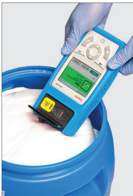
The analyzer performs identification through sealed packaging to minimize the risk of contamination and exposure.
