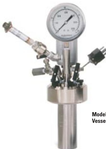
Model 4593 Reactor, Moveable Vessel, 100 mL, with PTFE Compression Gasket, and Split Ring Closure
