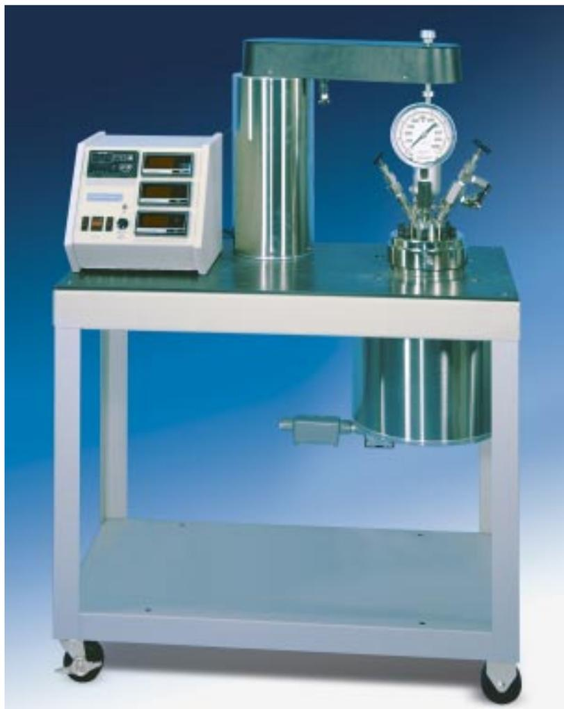
Model 4546C Reactor, 1200 mL, Moveable Head Style, on a Moveable Cart
