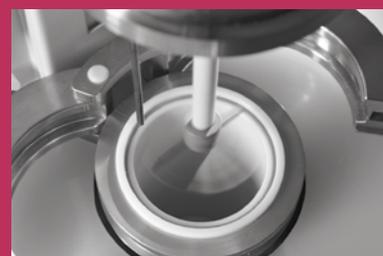
The synthWAVE features a powerful stirrer, which ensures vigorous stirring in the 1L PTFE vessel, or in all vials whenever a rack is used, thus assuring reliable and consistent results.
