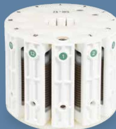
accessories are available to further expand the ETHOS UP capabilities: additional digestion rotors, inserts and micro-inserts to reduce blanks in the digestion processes, a dedicated configuration for total fat determination in food samples which greatly improves turn-around-time, and an ashing accessory which converts the digestion system into a microwave muffle.
