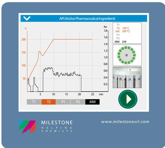
*easyTEMP temperature control of an exothermic reaction during the digestion of an API with HNO<sub>3</sub> and HCl in the SK-15 rotor*
