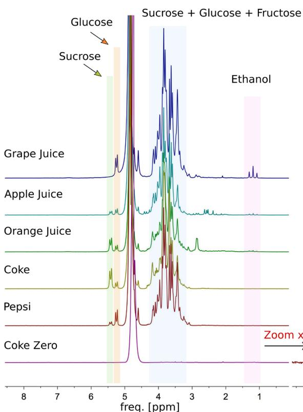
The Spinsolve 60 ULTRA was used to determine the sugar type and content present in soft beverages. The high sensitivity of the system allows you to quantify with high accuracy the concentration of several components like ethanol typically present at very low concentrations in natural fruit juices. These spectra were collected in 8 min., except the Coke Zero was acquired in 1 hour.
