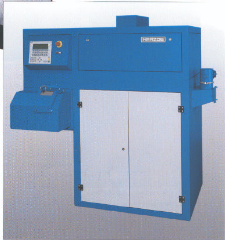
UNIVERSAL SAMPLE PREPARATION FOR SPECTRO- CHEMICAL ANALYSIS: HERZOG AUTOMATIC GRINDER AND MILLER FOR STEEL AND IRON SAMPLES
