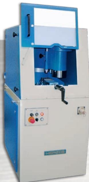
HPF with manual clamping device
