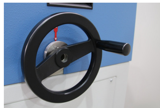
Precise adjustment of the milling depth
