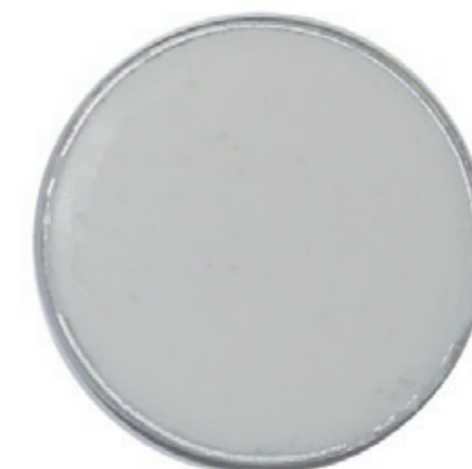
Pressed tablet, made by pressing in an aluminium tray
