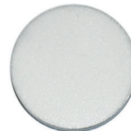
Pressed tablet, made by free pressing
