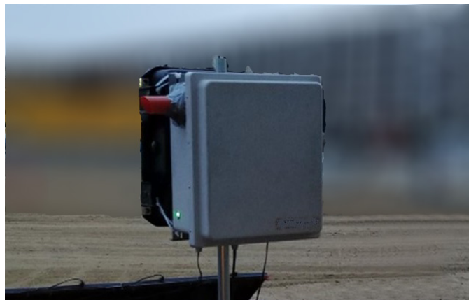
Figure 2: VOCAM is shown integrated with sensors for wind-speed, direction, and total VOCs.
