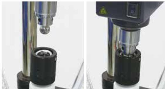
AGI designed Flexible Bearing Coupling creates flexibility between the motor and stir shaft allowing for efficient stirring even if the motor and connection is not aligned perfectly.
