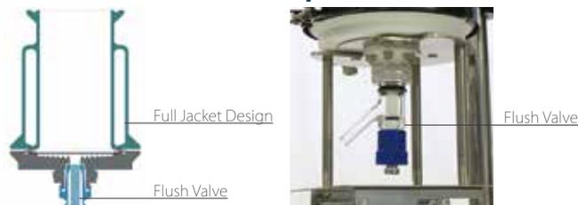
Heat transfer fluid runs from top to bottom.
