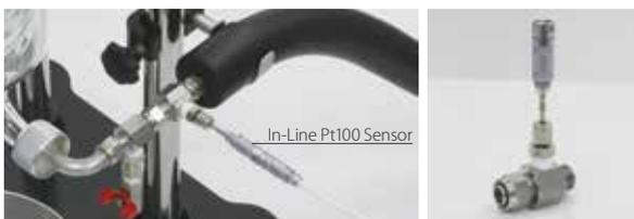
Temperature can be measured at either or both inlet and outlet.
