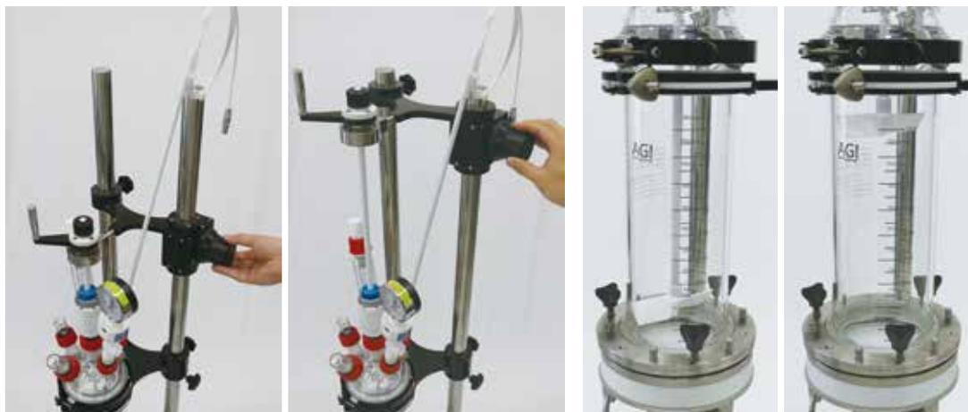
Lower and lift the shaft easily using one hand. This allows for easy simple height adjustment for stirring shaft.
