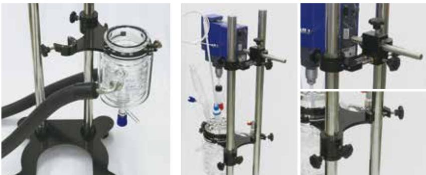
Allows for easy access for cleaning. Simply adjust the knob to release vessel and motor.
