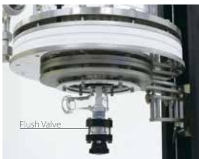
Heat transfer fluid runs from top to bottom. Flush Valve minimizes dead space.
