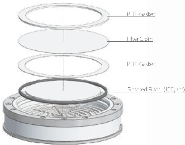
Separated Filter Components and Filter Cloth placement.
