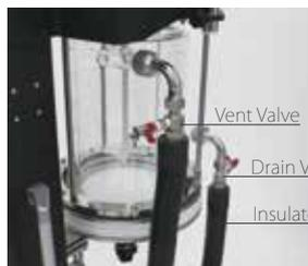
Vent Valve and Drain Valve allows for quick and easy drainage.
