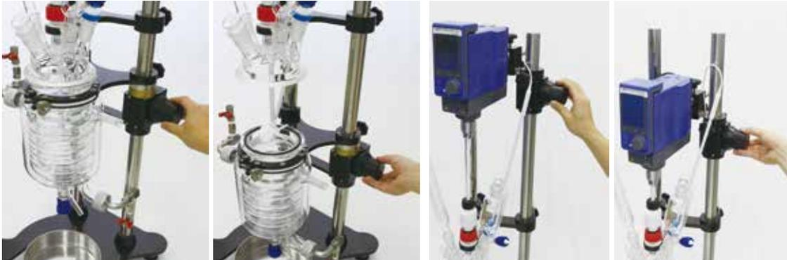
Easy lowering/lifting with single handed operation for motor and vessel. This allows for easy assembly and cleaning.
