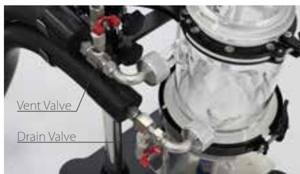
Quick and easy to drain thermal fluid.
