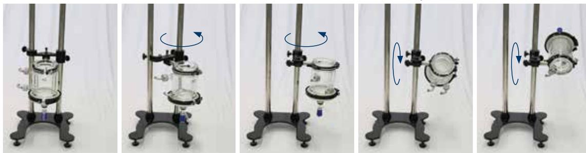
360° rotation allows for easy removal and cleaning.
