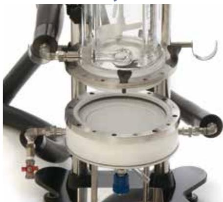
Liquid heated filter housing allows for drying of cake.
