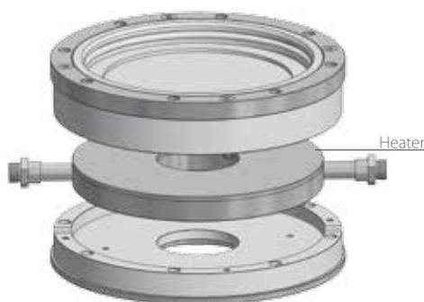
Separated Filter Dryer Components.
