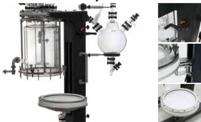
Operator can adjust and align the filter unit without tools. You need not make frequent filter adjustments. The swinging mechanism helps with filter access, and you can retrieve the cake easily.
