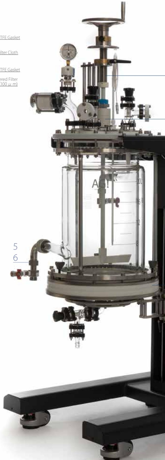
Operator can adjust and align the filter unit without tools. You need not make frequent filter adjustments. The swinging mechanism helps with filter access, and you can retrieve the cake easily.
